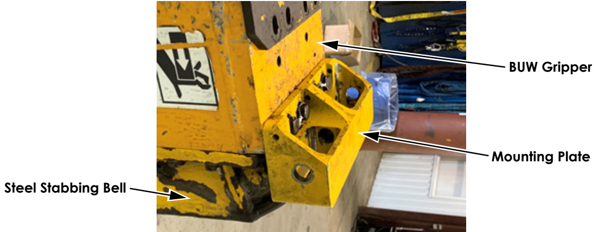
Figure 2: Mounting plate (Canrig P/N: DT24188) installed on top drive
