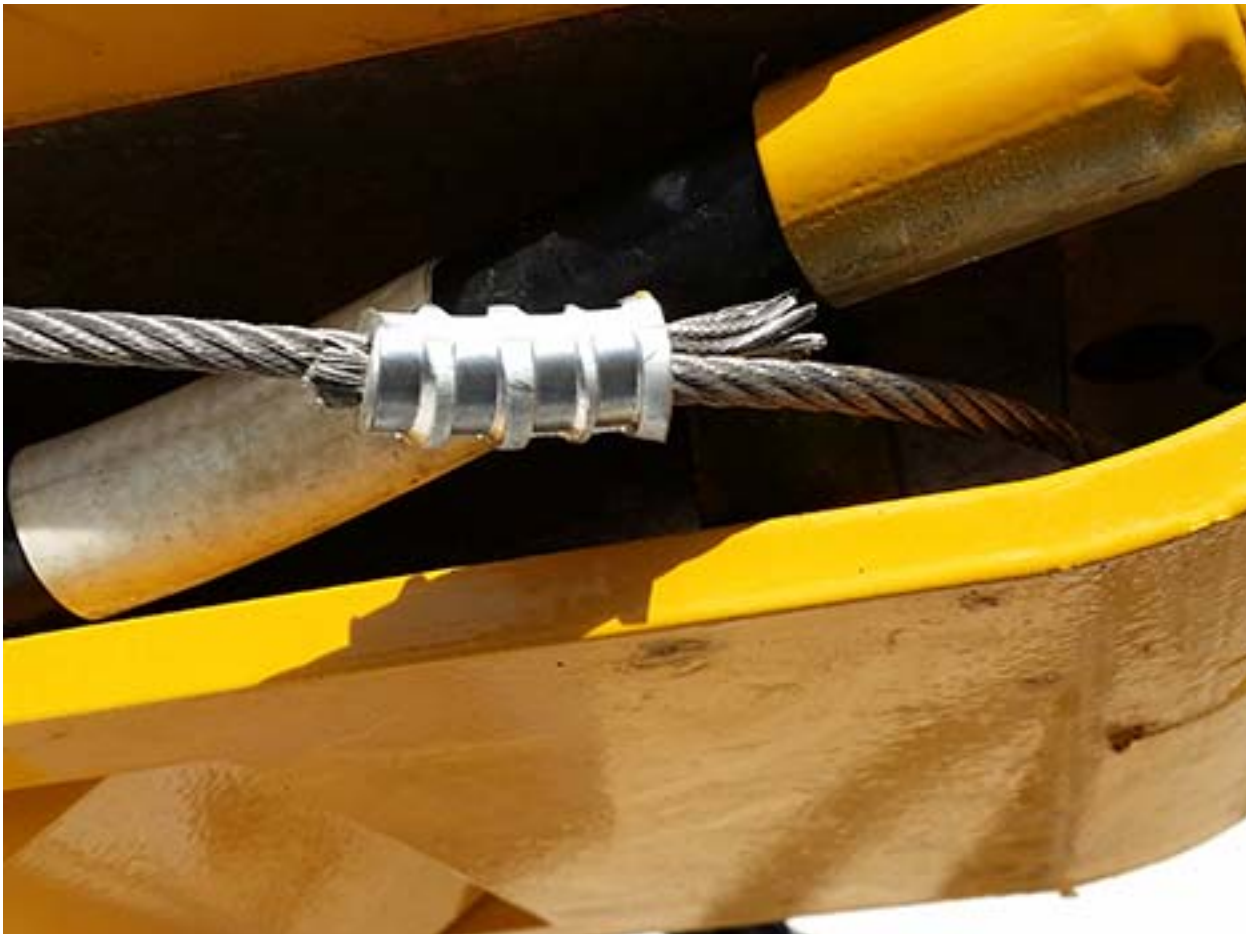
Figure 7: Safety wire crimped in the ferrule.
