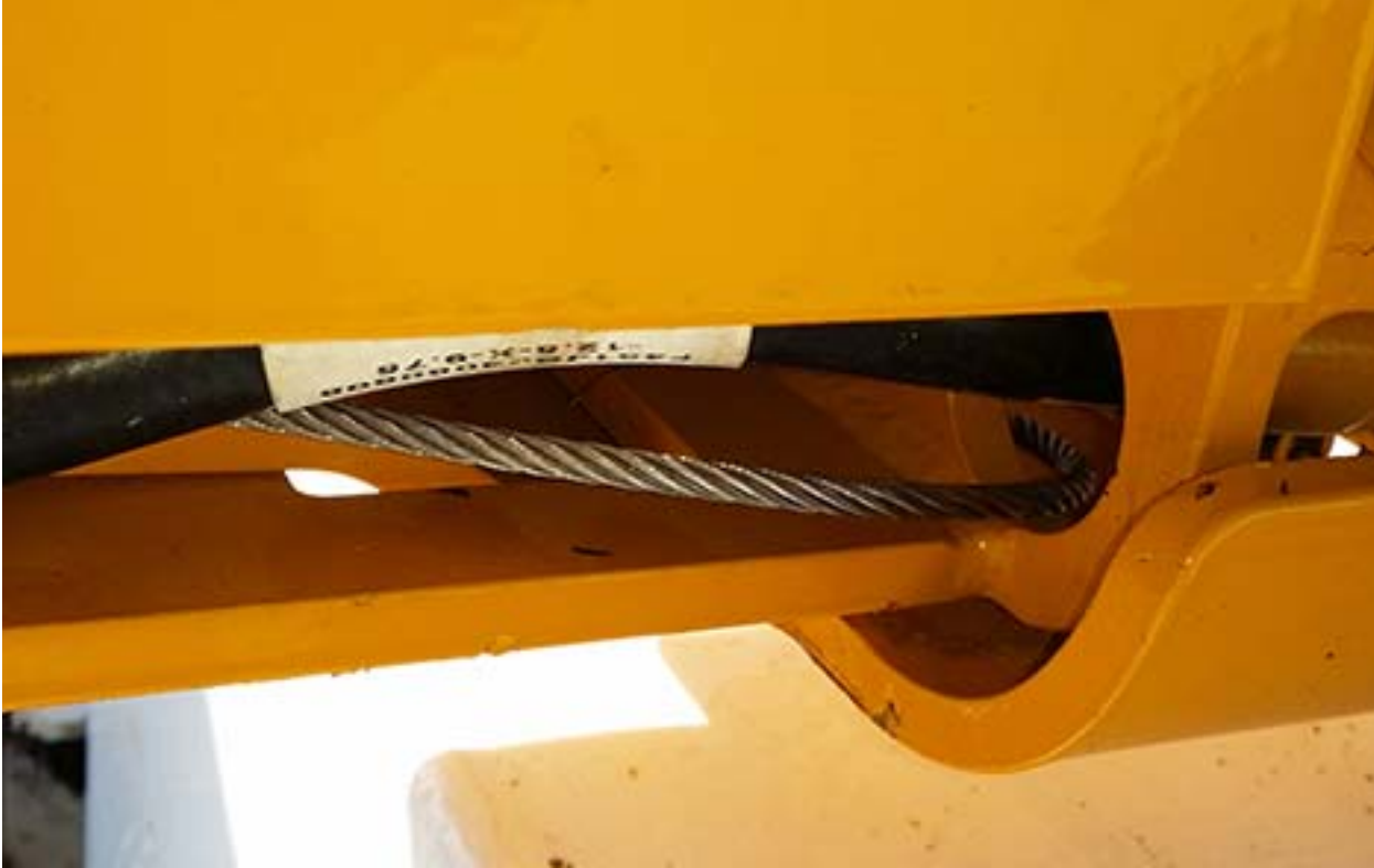
Figure 4: Pass the safety wire through the hole with the hydraulic hose.
